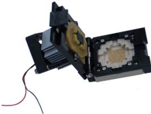
Above: Yamaichi BGA Test Contactor With Integral Heatsink and Fan
